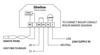
LS & LR ARE NORMALLY THE ROOM THERMOSTAT CONNECTIONS
